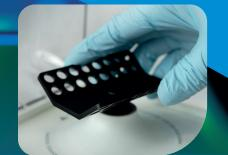
Rotor exchange is quick and easy - just lift off and push on - and requires no tool for you to lose or have to find each time you want to change sample size
